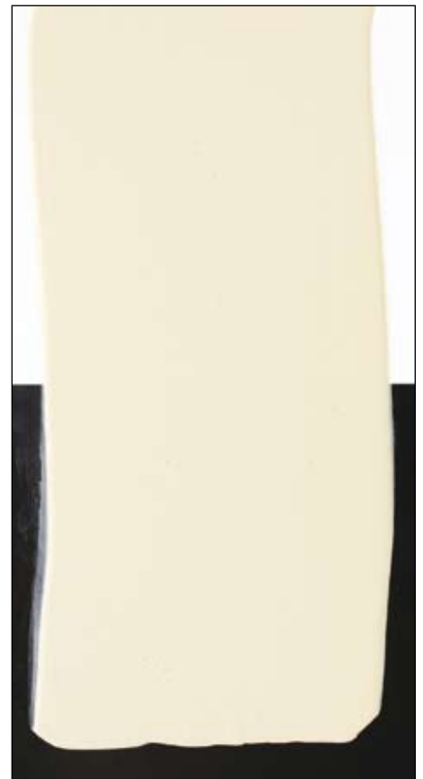
Reached opacity: 225 \mu\text{m} wet film (160 DFT). Jotacote Universal Buff example.
