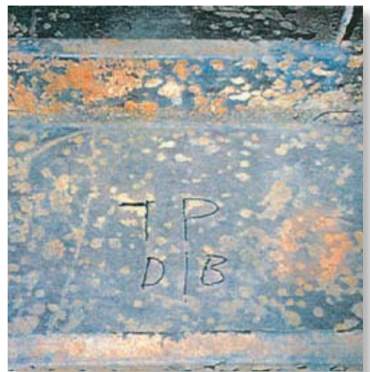
Majority of blisters have been noted and broken with waterjetting – no evidence of pitting.
