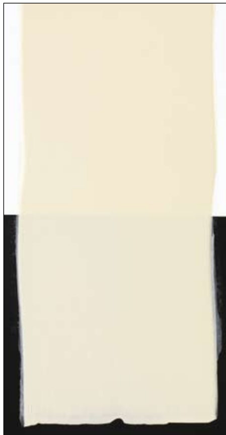
Not reached opacity: 140 \mu\text{m} wet film (100 DFT). Jotacote Universal Buff example.
