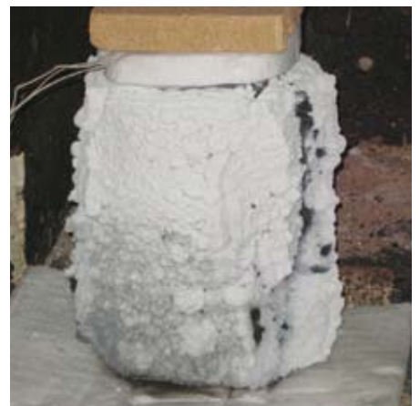
Heated steelwork producing char
